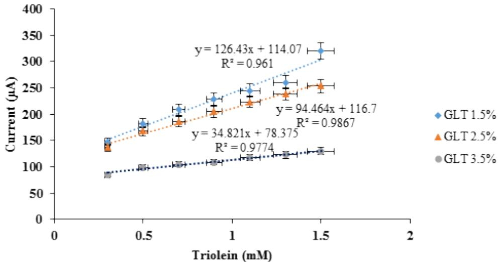
Figure 3. The effect of glutaraldehyde content on biosensor response.
