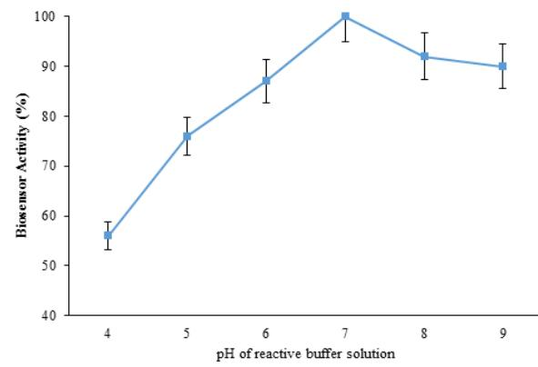
Figure 4. The effect of pH on biosensor response.
