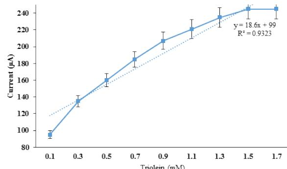
Figure 5. Calibration curve for the developed biosensor.
