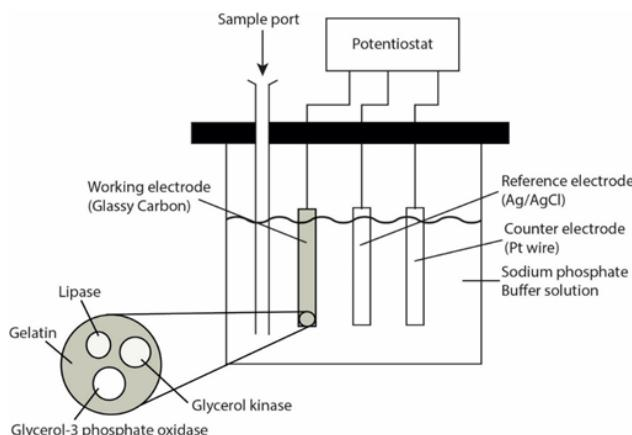
Figure 1. Schematic diagram of the biosensor.
